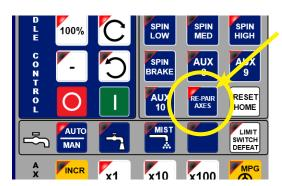
Push to "Re-Pair" the axes after an Estop condition during homing cycle before jogging the gantry!! LED turns green and label changes to let you know that the axes are paired.
