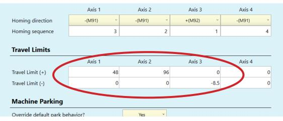
Re-enter Travel limit values or use "restore report" in CNC12 utility menu to restore values automatically after an Estop condition during the master/slave axis independent movement stage.
