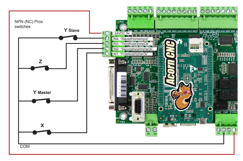
Either of these input assignments will work with this wiring configuration above.
