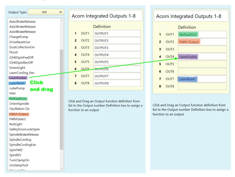
For preset Laser setups, like J tech schematics <u>S15049</u>, <u>S15056</u>, and <u>S15057</u>, the Wizard will place the Laser outputs in their appropriate slots automatically. To assign them yourself, simply click and drag the outputs into the desired output slots.
