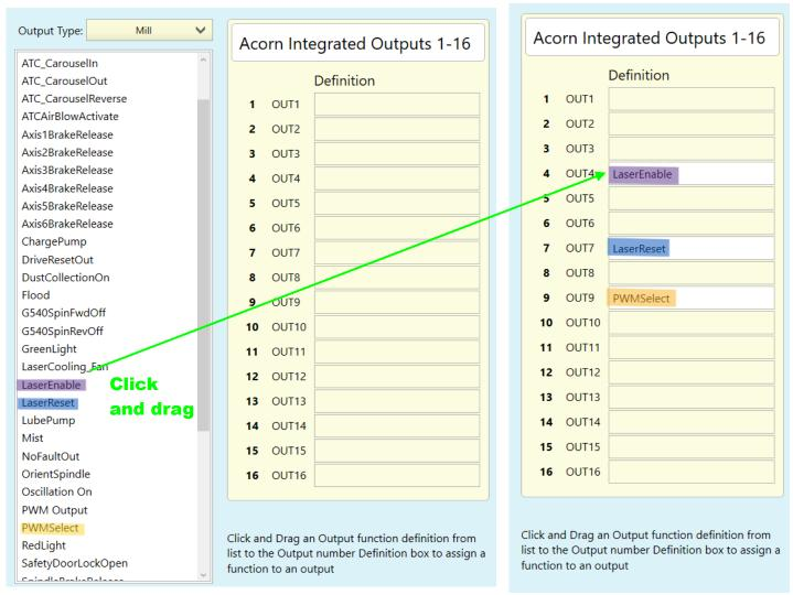
The AcornSix wizard also handles preset J tech Laser setups listed on the PWM Setup tab automatically. For custom Laser setups, click and drag the outputs to the desired output slots.
