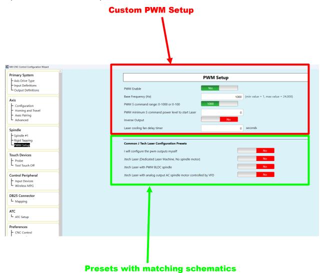
When using one of the presets **be sure to follow the corresponding hookup schematic exactly** as these presets configure the Acorn Wizard inputs and outputs to match the schematic!
