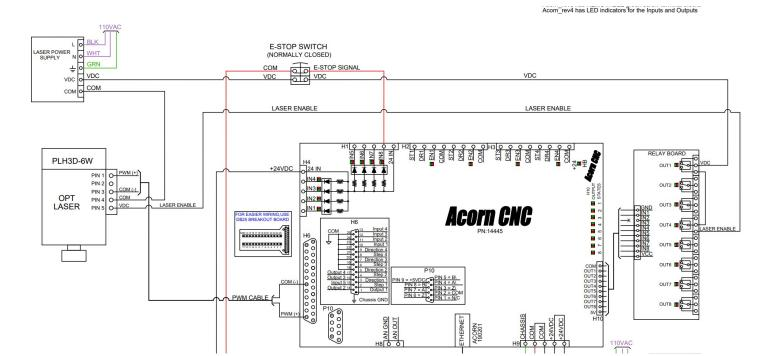
**AcornSix Example Hookup:** Using AcornSix schematic <u>S15217</u> NEJE Laser as an example, follow these steps for setting up a Laser using the AcornSix Wizard.
