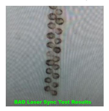
As you can see, the dots are not aligned down the axis, which shows that the machine has backlash in the X axis and is losing motion when changing directions. Since each "dot" is 0.006 inches long we can make an educated guess at the backlash adjustment need to align the "dot"
